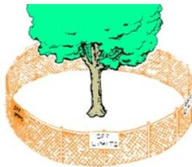
**Figure 2.** Set up signs and fences around trees to be protected from construction.
