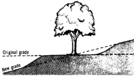
**Figure 6.** Using fills and cuts to improve PRZ for a tree on a slope.
